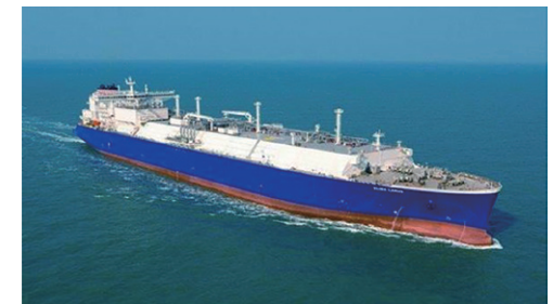
Liquefied gas carrier equipped with a dual-fuel engine that can also use gas fuel to reduce environmental impact (France LNG Shipping S.A.S)
